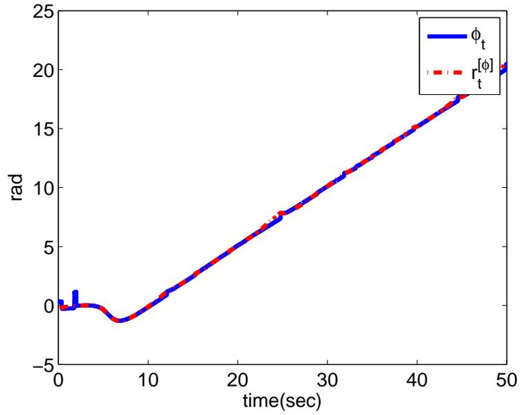
Fig. 7. Solid line: The orientation of the autonomous vehicle ( $\phi_t$ ). Dashed line: The desired orientation  $r_t^{[\phi]}$  for the case, where the communication is subject to 90 percent packet dropout ( $\alpha = 0.9$ )
