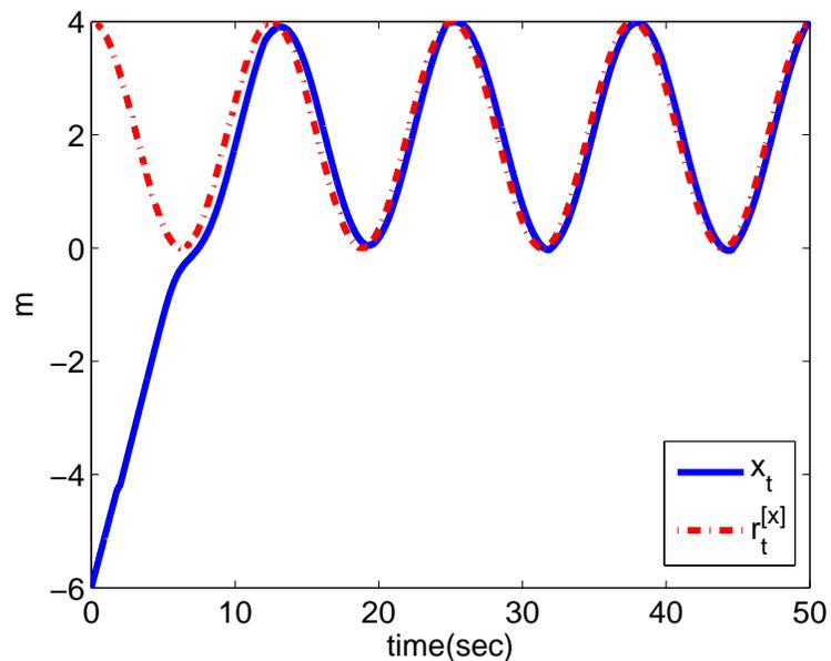
Fig. 5. Solid line: The  $x_t$  position of the autonomous vehicle. Dashed line: The desired position  $r_t^{[x]}$  for the case, where the communication is subject to 90 percent packet drop out (i.e.,  $\alpha = 0.9$ )
