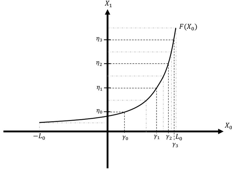
Fig. 3. Equal sized, non-overlapping sub-intervals for encoding with the rate  $R = 2$
