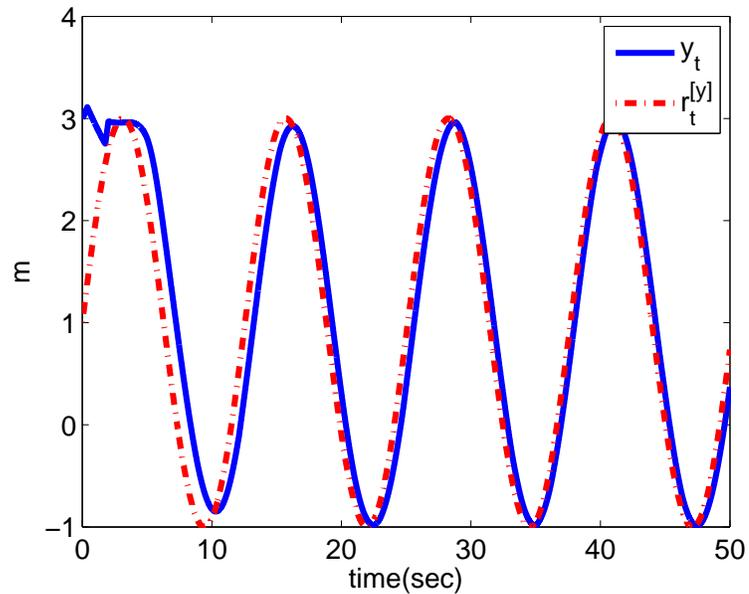
Fig. 6. Solid line: The  $y_t$  position of the autonomous vehicle. Dashed line: The desired position  $r_t^{[y]}$  for the case, where the communication is subject to 90 percent packet dropout (i.e.,  $\alpha = 0.9$ )
