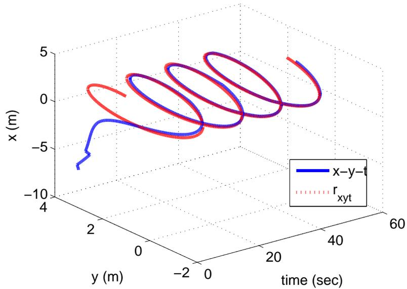
Fig. 8.  $x_t - y_t - time$  diagram for the case where the communication is subject to 90 percent packet dropout ( $\alpha = 0.9$ ). Solid line:  $x_t - y_t - time$  diagram of the autonomous vehicle. Dashed line: The desired  $r_{xyt}$
