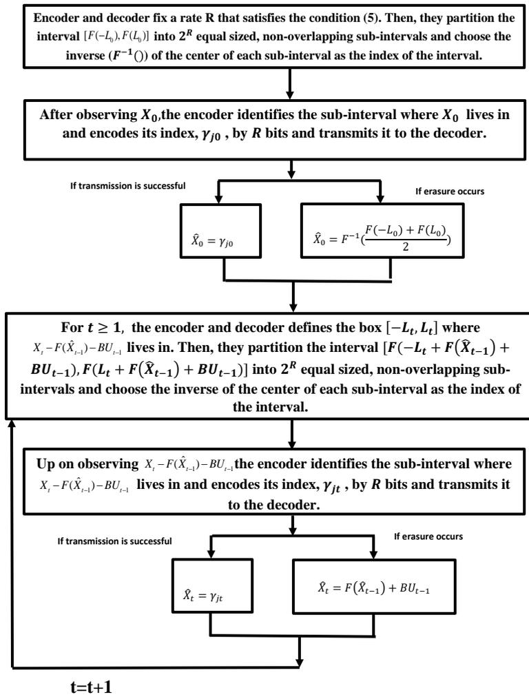
Fig. 2. The proposed coding algorithm for the scalar case
