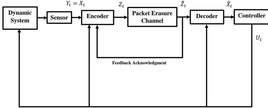
Fig. 1. A dynamic system controlled over the packet erasure channel with feedback acknowledgment
