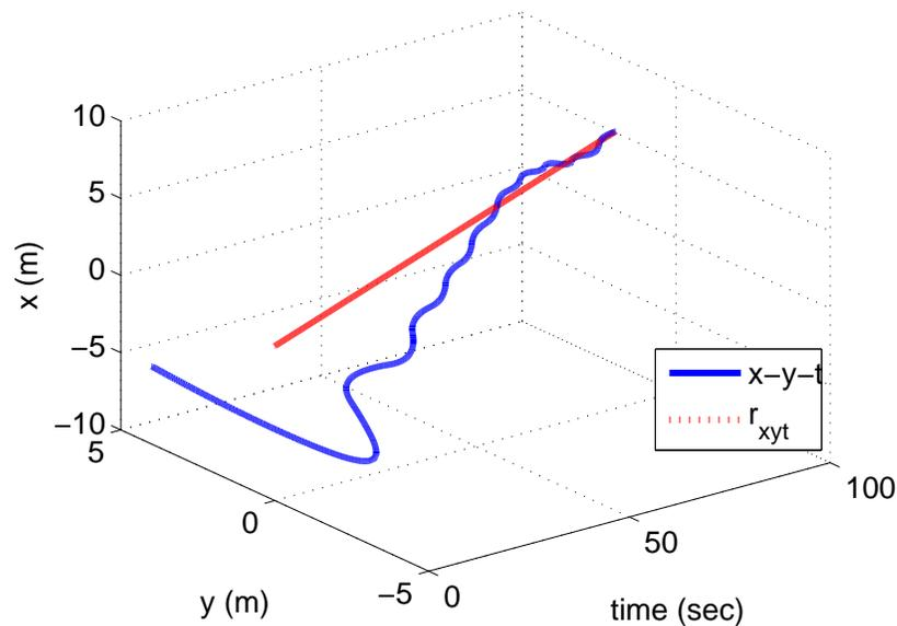
Fig. 12.  $x_t - y_t - time$  diagram for the case of  $\alpha = 0.9$  when the feedback linearization technique of [20] is used for tracking a straight line
