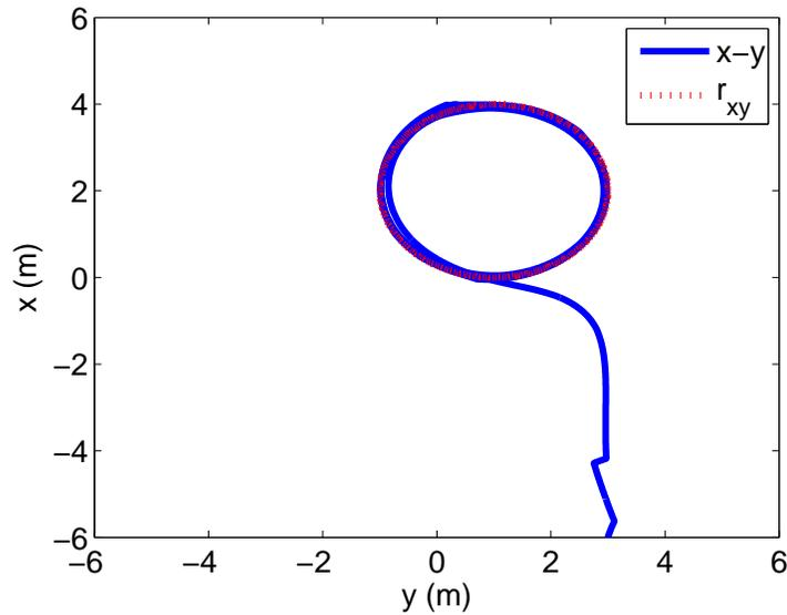
Fig. 9.  $x_t - y_t$  diagram for the case where the communication is subject to 90 percent packet dropout ( $\alpha = 0.9$ ). Solid line:  $x_t - y_t$  of the autonomous vehicle. Dashed line: The desired  $r_{xy}$
