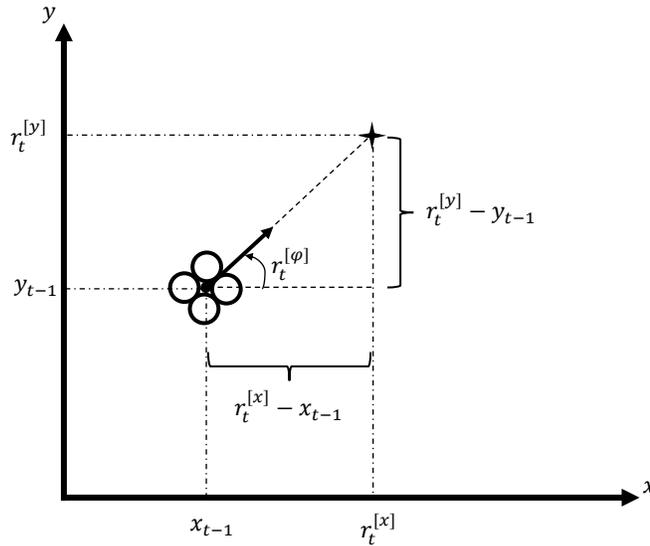
Fig. 4. An autonomous vehicle with the positions  $x_{t-1}$  and  $y_{t-1}$  moving toward the desired positions  $r_t^{[x]}$  and  $r_t^{[y]}$ , respectively
