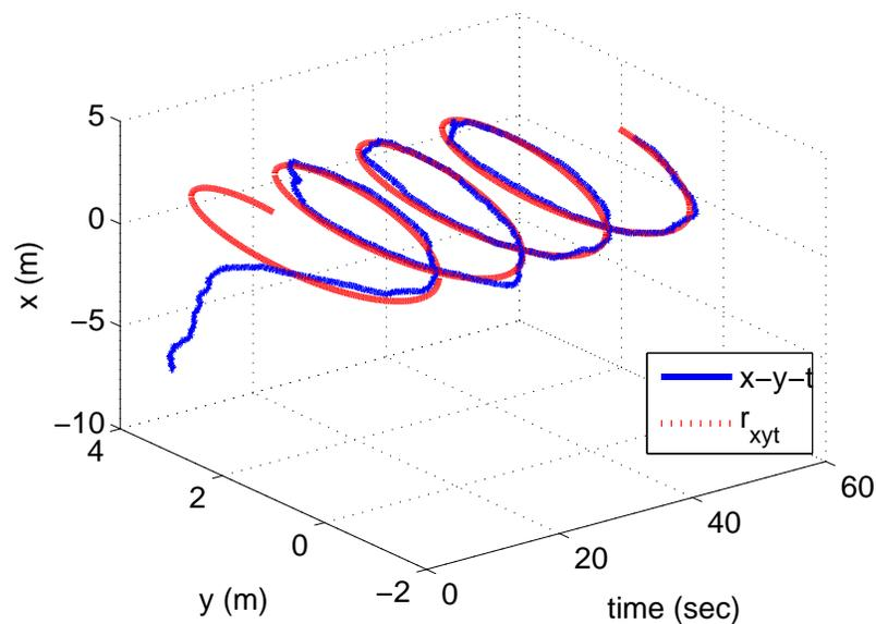
Fig. 10.  $x_t - y_t - time$  diagram for the case where the communication is subject to 90 percent packet dropout ( $\alpha = 0.9$ ) and the unicycle model is subject to process noise. Solid line:  $x_t - y_t - time$  diagram of the autonomous vehicle. Dashed line: The desired  $r_{xyt}$
