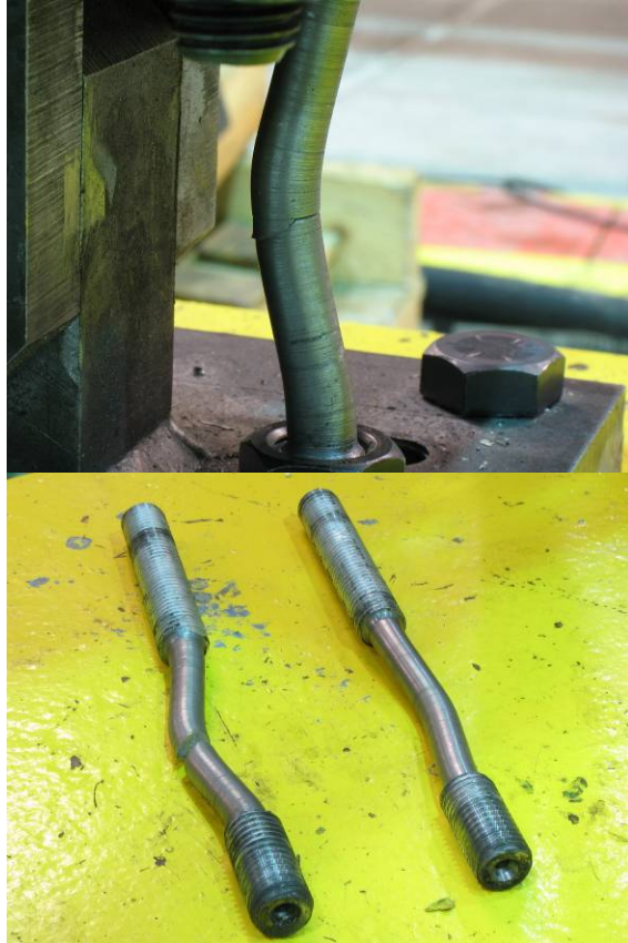
Figure 6-19 Fractured coupon during an experiment.
