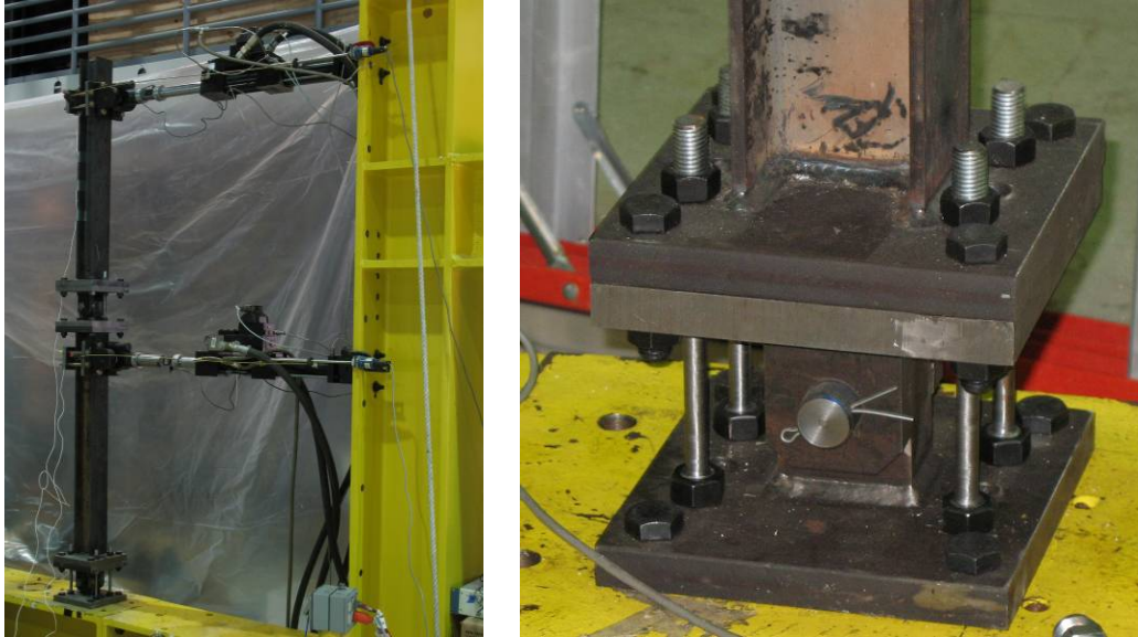
Figure 3-3 Pictures of two-degree-of-freedom test setup and the lower clevis.
