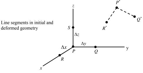
We are interested in the projection of  $\overline{P^*R^*}$  and  $\overline{P^*Q^*}$  on to the *xy* place (on to the place the line segments were in undeformed state)
