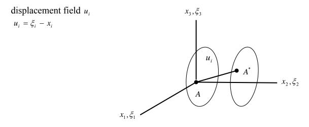
We may express  $u_i$  as a function of Lagrange coordinate  $x_i$ , in which case it expresses the displacement from the position  $x_i$  in the undeformed state to the deformed position  $\xi_i$ .
