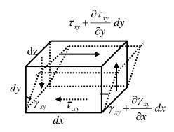
$$\begin{bmatrix} \left(\tau_{xy} + \frac{\partial \tau_{xy}}{\partial y} \, dy\right) dz dx \end{bmatrix} \left\{ d \left(\gamma_{xy} + \beta \frac{\partial \gamma_{xy}}{\partial x} \, dx\right) dy \right\}$$
