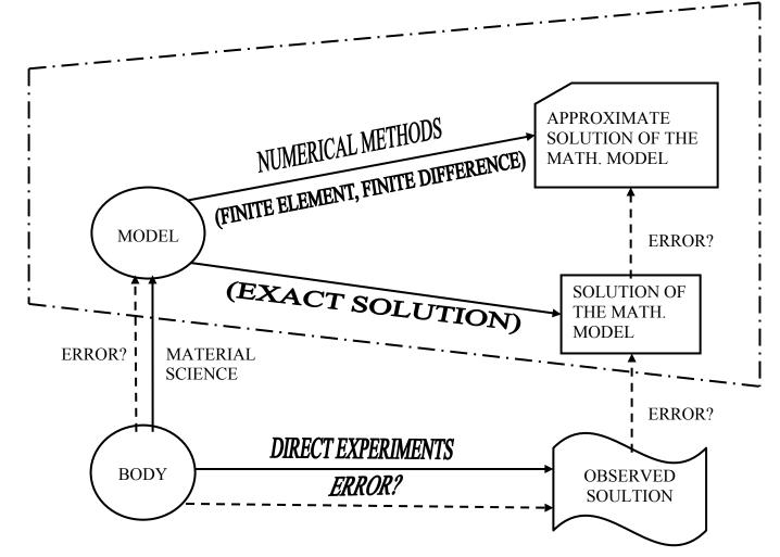
Model studies or direct experiment include checking of the approximate solution with the state variables in laboratory which involves dimensional analysis and similitude.
