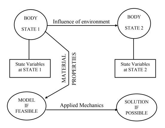
State variables involve displacements, velocities, pressure, temperature, stress, strain, charge, position, etc.
