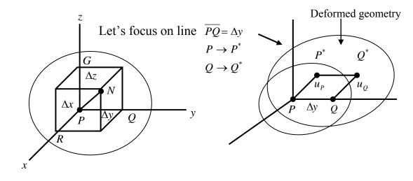
Projection of  $\overline{P^*Q^*}$  in the y direction  $(\overline{P^*Q^*})_y$  $(\overline{P^*Q^*})_y = \Delta y + (u_y)_Q - (u_y)_P$
