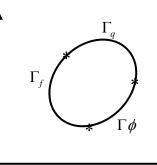
$$\delta J = \int_{\Omega} \left[ k \,\phi_x \,\delta\phi_x + k \,\phi_y \,\delta\phi_y - Q \,\delta\phi \right] d\,\Omega - \int_{\Gamma_q} \overline{q} \,\delta\phi \,d\,\Omega$$
