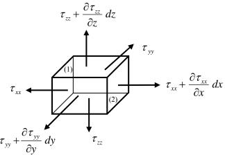
The displacements of faces 1 and 2 in the x direction are  $u_x$  as  $u_x + \frac{\partial u_x}{\partial x} dx$ , Increment of mechanical work done by the stresses on the element during deformations is:
