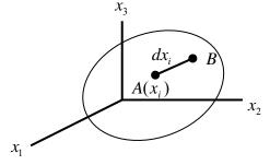
Line segment in the undeformed geometry
