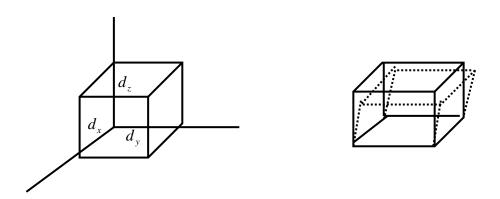
Zero shear stress means side will remain orthogonal on deformation. However position and orientation of the element may change as length of the sides and volume.
