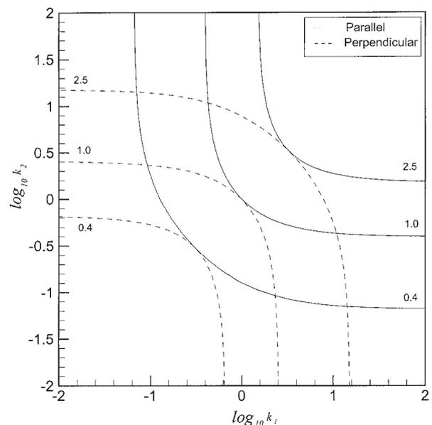
**Figure 3.** The contours of the effective conductivity in the parallel and perpendicular directions for the case of equal sized cylinders.  $f_1 = 0.4$ ,  $f_2 = 0.4$  and  $b = \sqrt{3}$ .
