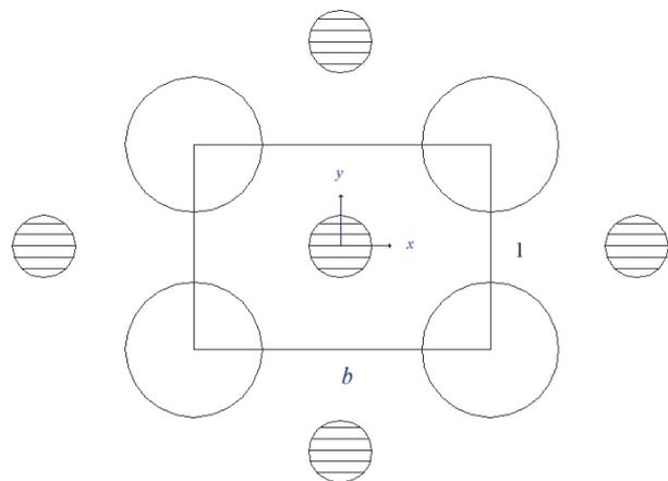
**Figure 1.** The unit cell of the three-phase composites under study. Cylinders of the same type have a distance equal to a unity in the  $x$ -direction and  $b$  in the  $y$ -direction.
