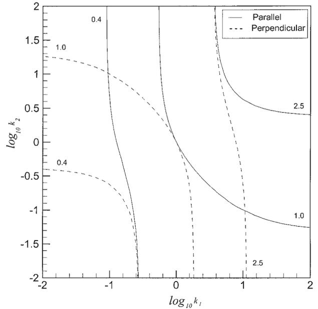
**Figure 5.** The contours of the effective conductivity in the parallel and perpendicular directions for the case of unequal sized cylinders.  $f_1 = 0.4$ ,  $f_2 = 0.2$  and  $b = \sqrt{3}$ .
