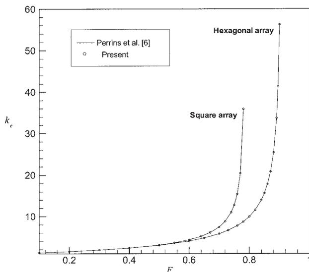
**Figure 2.** The effective conductivity of two-phase composites with mono-sized perfectly conducting circular cylinders arranged in square and hexagonal orders.  $F$  shows the volume fraction of the cylinders. The solid lines are the results of Perrins *et al* [6] and the dotted lines are those obtained by solving the governing equations of the three-phase composites.
